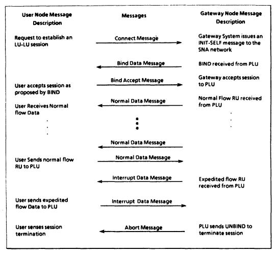
Figure 6-7: SNA Gateway Access Message Exchange
