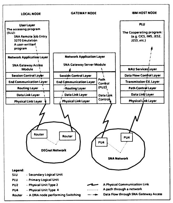
Figure 6-8 depicts the relationship of these modules to the SNA network and to the IBM host application (the PLU):
