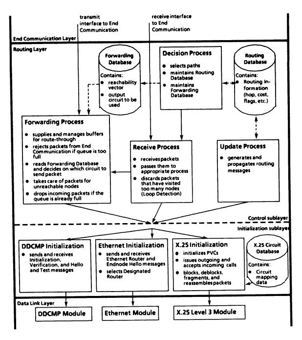
Figure 3-4: Routing Layer Components and their Functions
