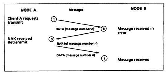
Figure 2-5: DDCMP Message Exchange, Showing Error Recovery
