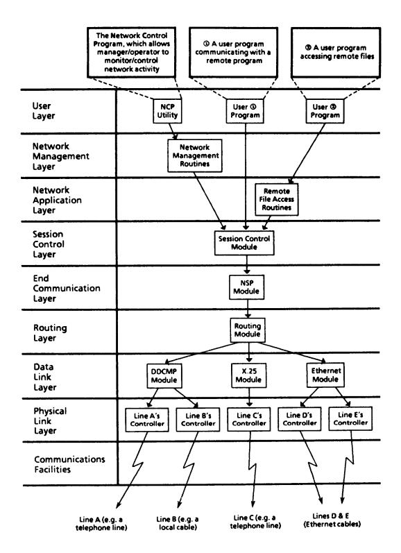
Figure 1-3: DNA Modules Resident in a Typical DECnet Node
