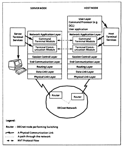
Figure 6-3: Network Virtual Terminal Service
