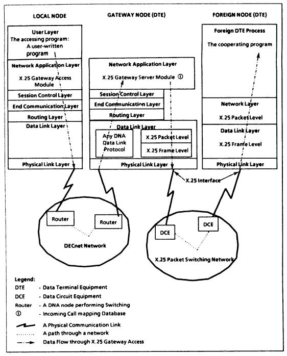
Figure 6-6: X.25 Gateway Access Operation
