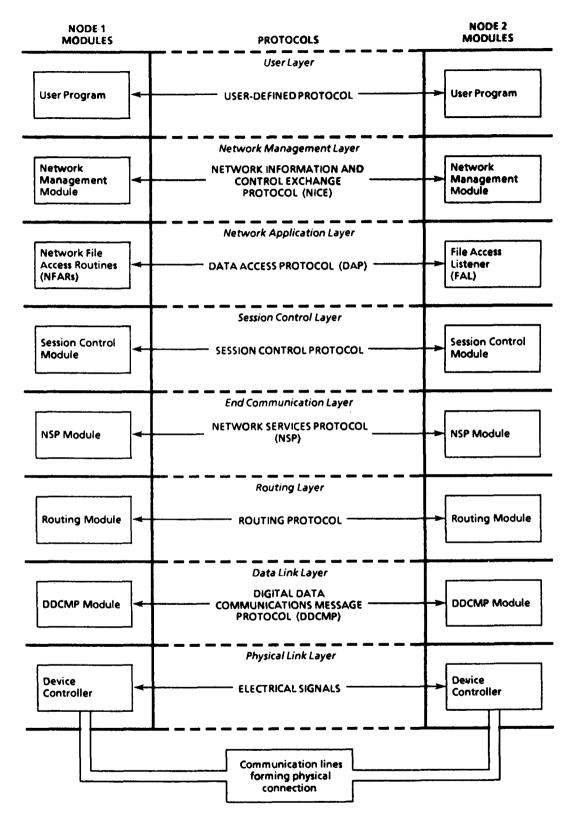
Figure 1-4: Protocol Communication between Two Nodes
