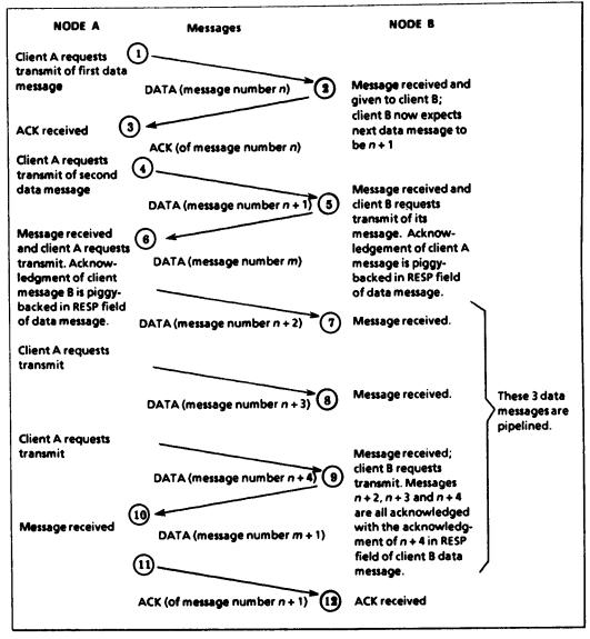
Figure 2-4: Typical DDCMP Message Exchange, Showing Positive Acknowledgment, Piggybacking, and Pipelining
