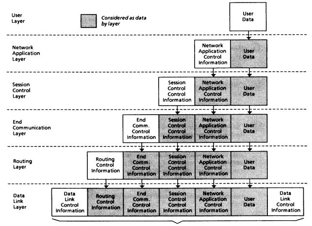
Complete Envelope Transmitted from One Node to an Adjacent Node
