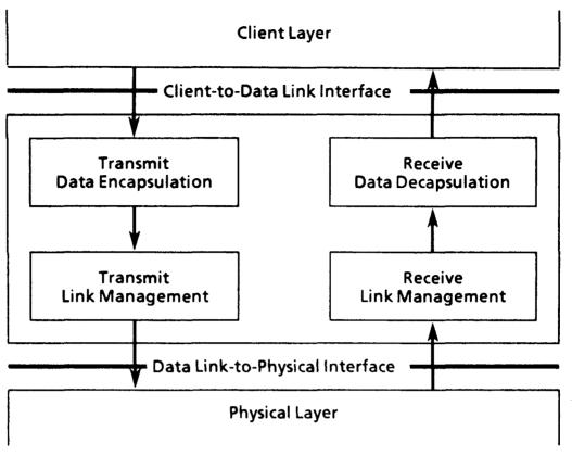
Figure 2-6: Ethernet Data Link Layer Functions
