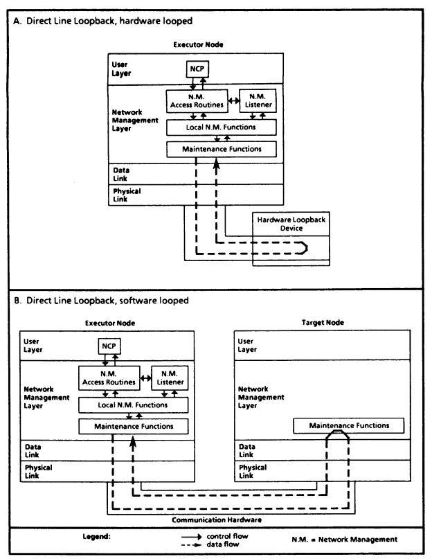
Figure 7-3: Line Loopback Tests
