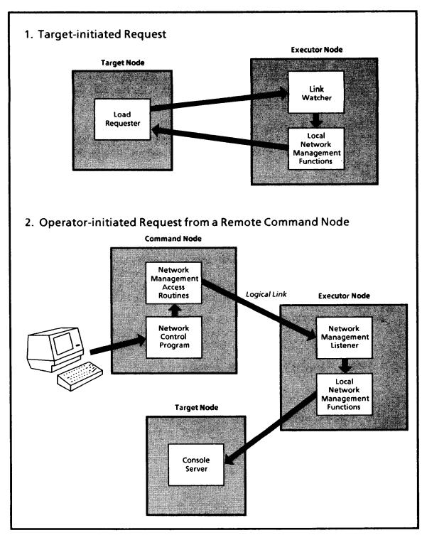
Figure 7-2: Down-Line Load Request Operation
