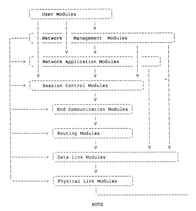
Horizontal arrows show direct access for control and observation of parameters, counters, etc. Vertical arrows show interfaces between layers for normal user operations such as file access, down-line load, and logical link usage.
