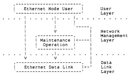
Arrows indicate flow of control. Vertical arrowheads indicate User Interfaces, horizontal arrowheads indicate Network Management Interfaces.
